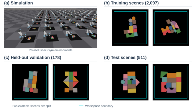
Fig. 4. Simulation setup and dataset. (a) Parallel Isaac Gym environments. (b)-(d) Representative training, validation, and test scenes (2,097/178/511); validation is used for model selection and the disjoint test set only for final evaluation.
